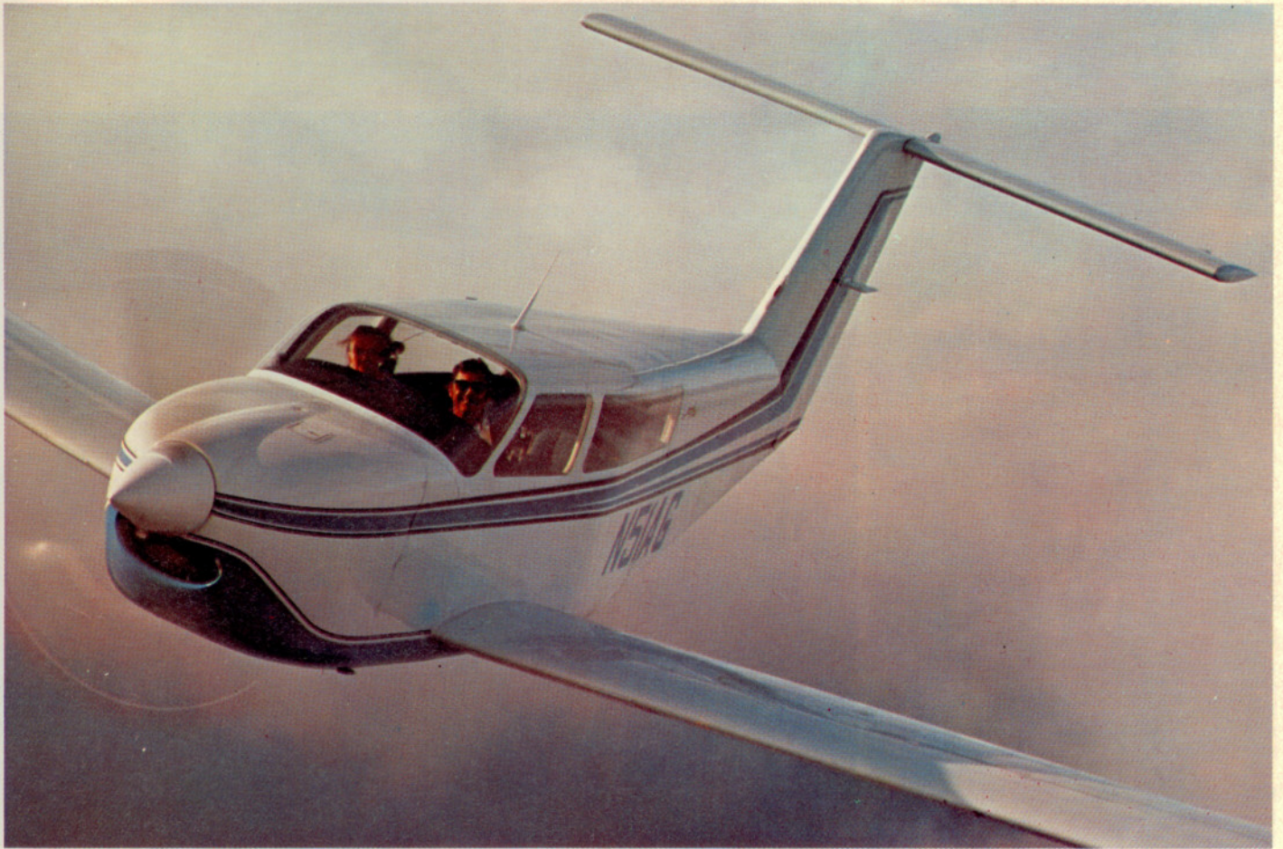
T-tail stabilator and angular shape characterize the new 217-mph, all-aluminum Bellanca. Flying is test pilot Jack Burden and designer Marvin Greenwood (right seat).
