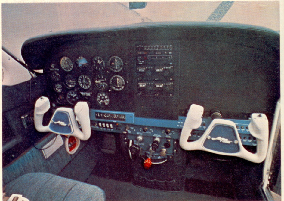
Instrument panel in the prototype is still a bit rough-edged, but shows how flight and engine instruments are all grouped in front of the pilot. Weather radar is being considered for right side.
