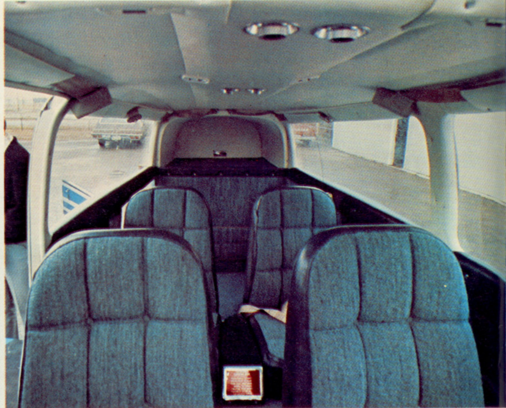
Long side windows and space between the seats give roomy feeling inside the Aries T-250. Emergency landing gear crank (left) is normally stowed between the two rear seats.
